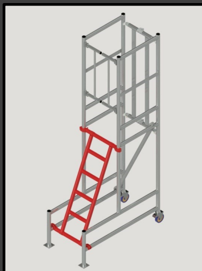
5 . Clip upper brace of the ladder above rings on the verticals with the assembled hooks at the top.
