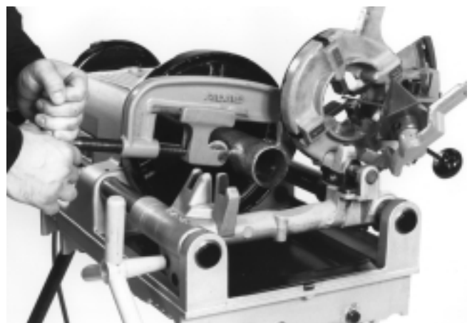
Figure 5 – Cutting Pipe with No. 763 Cutter
