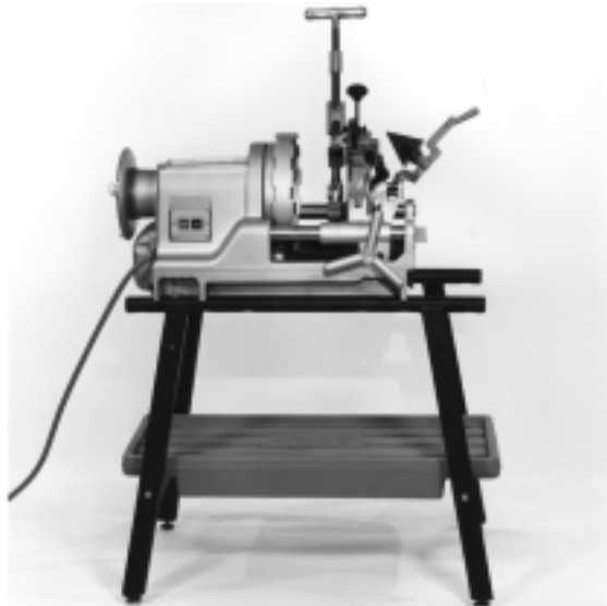
Figure 4 – Model 1233 Mounted on #100 Leg & Tray Stand
