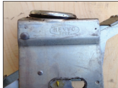
Top mounting plate distortion as a result of a single significant impact or multiple lower level impacts.
